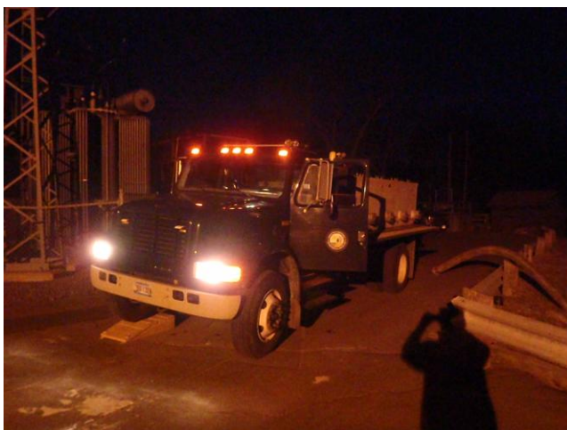
Releasing smolts into the Rainbow Dam tailrace. Note ramps to tilt truck toward the river to help drain the last of the water.
